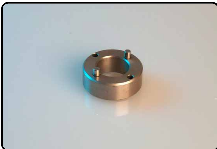
T145S Dis- / assembling tool screw-cap reservoir. With 2 pins d5x15 / T135. - All shock absorbers with reservoir.
